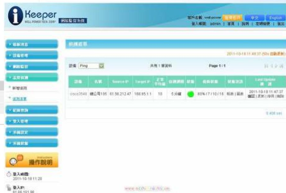
The screenshot shows the '偵測結果' (Detection Results) page. It displays a table of detection results for a 'Ping' test. The table has columns for '設備' (Device), '名稱' (Name), 'Source IP', 'Target IP', '正常平均值' (Normal Average Value), '偵測時間' (Detection Time), '狀態' (Status), '偵測結果' (Detection Result), '偵測時間' (Detection Time), and 'Last Update'.
