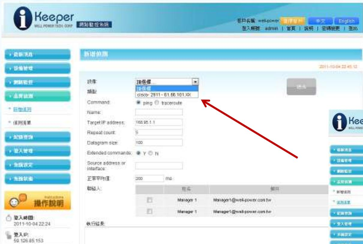
The screenshot shows the '新增偵測' (Add Detection) configuration page. A dropdown menu is open, showing 'ping' and 'traceroute' options. A red arrow points to the 'ping' option. Below the dropdown, the 'Command' field is set to 'ping', and the 'Target IP address' is '168.88.1.1'. The 'Repeat count' is 5 and 'Datagram size' is 100. The 'Normal average value' is 200 ms. The 'Contact person' table lists two entries for 'Manager 1' with email 'Manager1@well-power.com.tw'.
